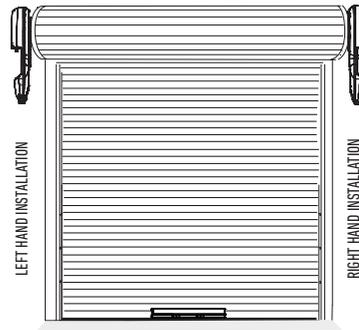
Minimum distance from edge of curtain to edge of door bracket 45 mm
